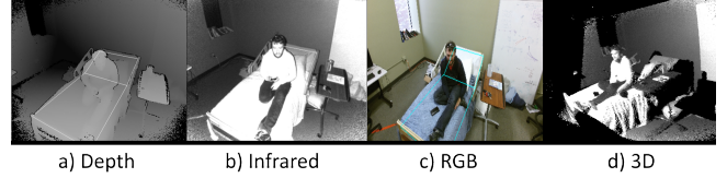
Figure 2. Image streams available from Kinect: a) depth, b) infrared and c) RGB. Image d) illustrates a 3D model of the scene that can be reconstructed from the depth information.
